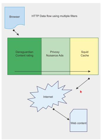
Figure 4. Data flow through the proxy
